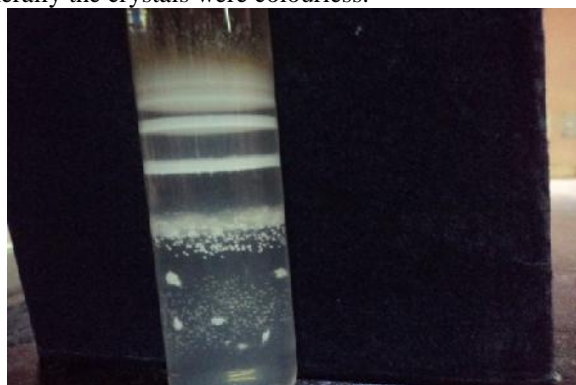
Fig.1 CHPD crystals grown in gel medium
