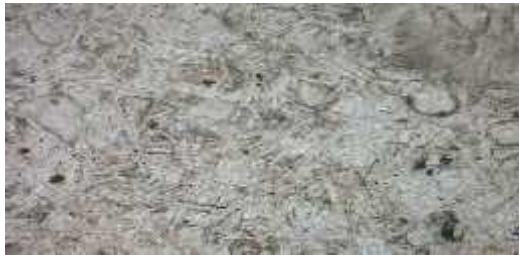
Figure3 Thin section of zeolite zk-5 (plain crosspolarized light)
