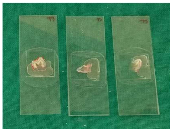
Fig 5 Slides preparation for viewing under confocal laser scanning microscope
