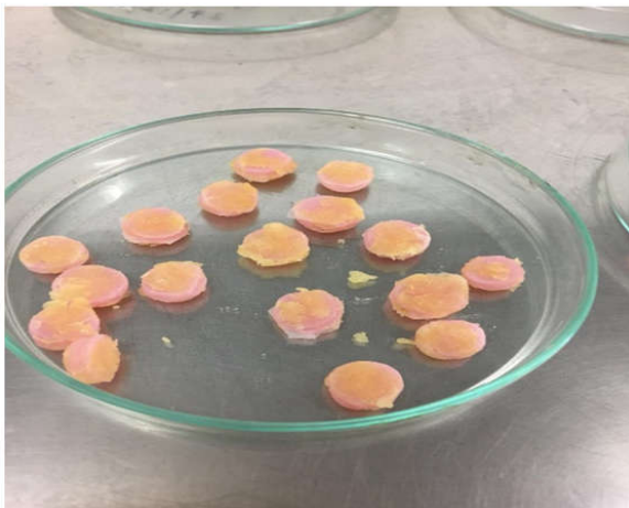
Fig 2 Acrylic disks coated with Nystatin incorporated denture adhesive
