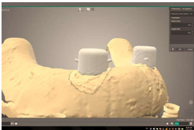
Fig 5 Planning the design of the secondary copings with mesial and distal projections
