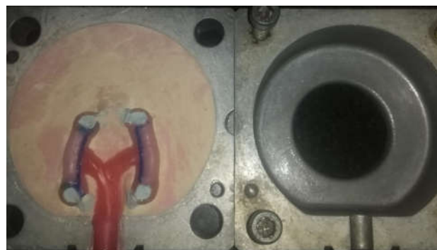
Fig 2 waxed frameworks were invested in a special flask
