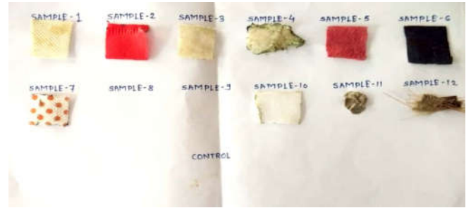
Fig 2 Samples of nonwoven bags after 30 days, when subjected for biodegradation in In- vitro condition.
