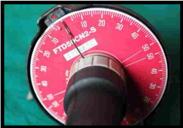
Figure 7 Round dial of the modified torque wrench device (FTD50CN2-S)
