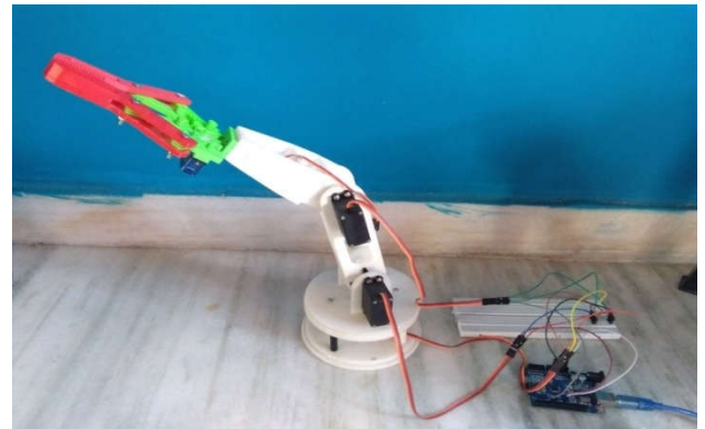
Figure 17 Full assembly of robotic arm
