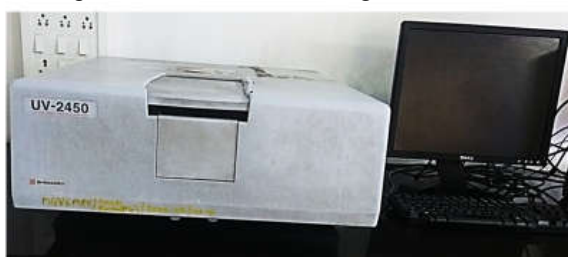
Figure 1 Spectrophotometer used in the study to determine the wavelengths of three dyes at varying concentrations.
