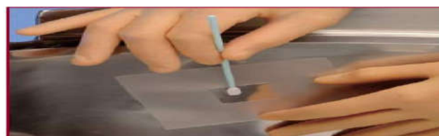
Figure 4 Texwipe swab swabbing on template
