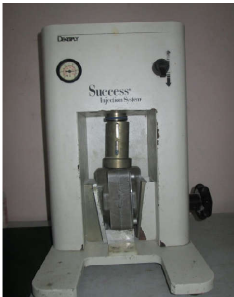
Fig 9 injection molding apparatus used for group B II samples.
