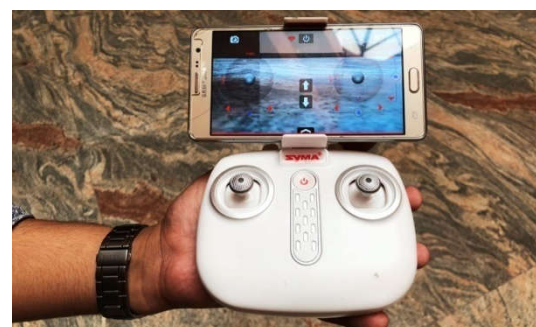
Figure 9 Video and photo transmission at ground station
