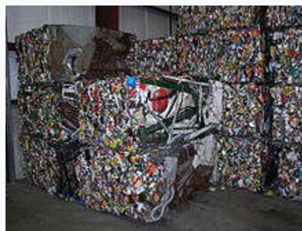
Steel crushed and baled for recycling
