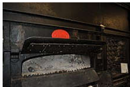
Manlove, Alliott & Co. Ltd. 1894 destructor furnace. The use of incinerators for waste disposal became popular in the late 19th century.
