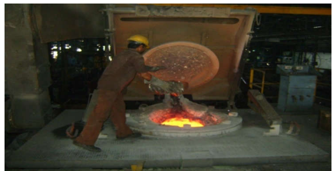
Fig 8 Labor loading scrap material in furnace
