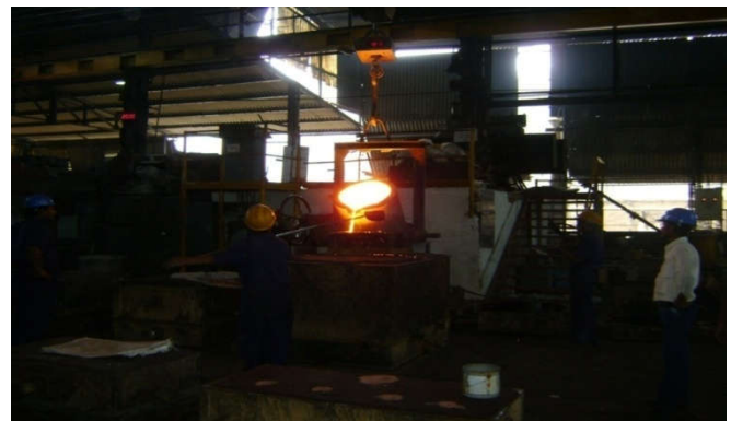
Fig 9 Molten metal's pouring in pallet
