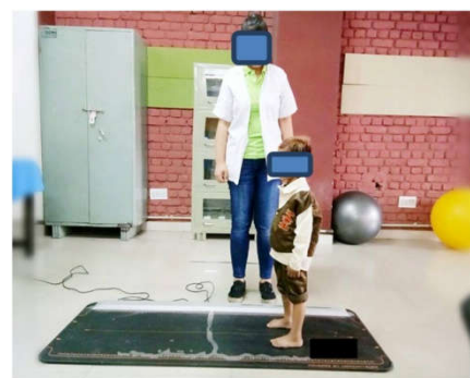
Figure 2 Subjects readings were taken on Win-Track Force Platform with eyes open while subject maintain the upright position and focusing on the target for 5 to 10 seconds (feet place side by side by forming an angle of 30 degrees with both heels separated by almost 4 cm).
