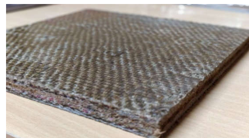
Figure 4 Coir based sandwich composite panel.
