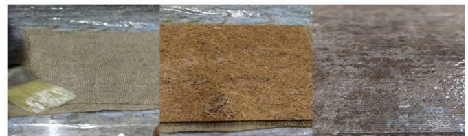
Figure 3 Sandwich samples manufacturing: Hand lay-up process
