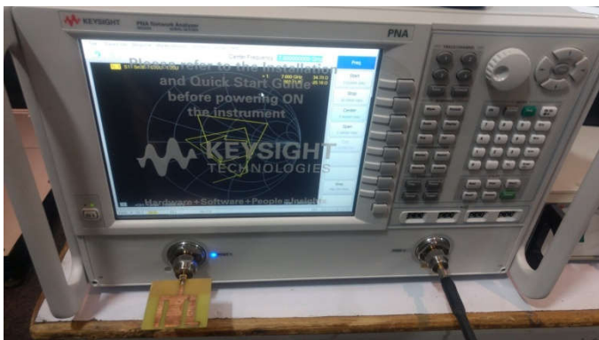
Fig 11 Measurement set up of VSWR & Input Impedance at 7GHz
