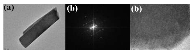
Fig 3 TEM images of \text{Sb}_2\text{S}_3 at 79 °C (a) nanorods obtain by solvothermal process after 6 hr. (b) SAED pattern of the nanorod and (c) HRTEM image of the nanorod.
