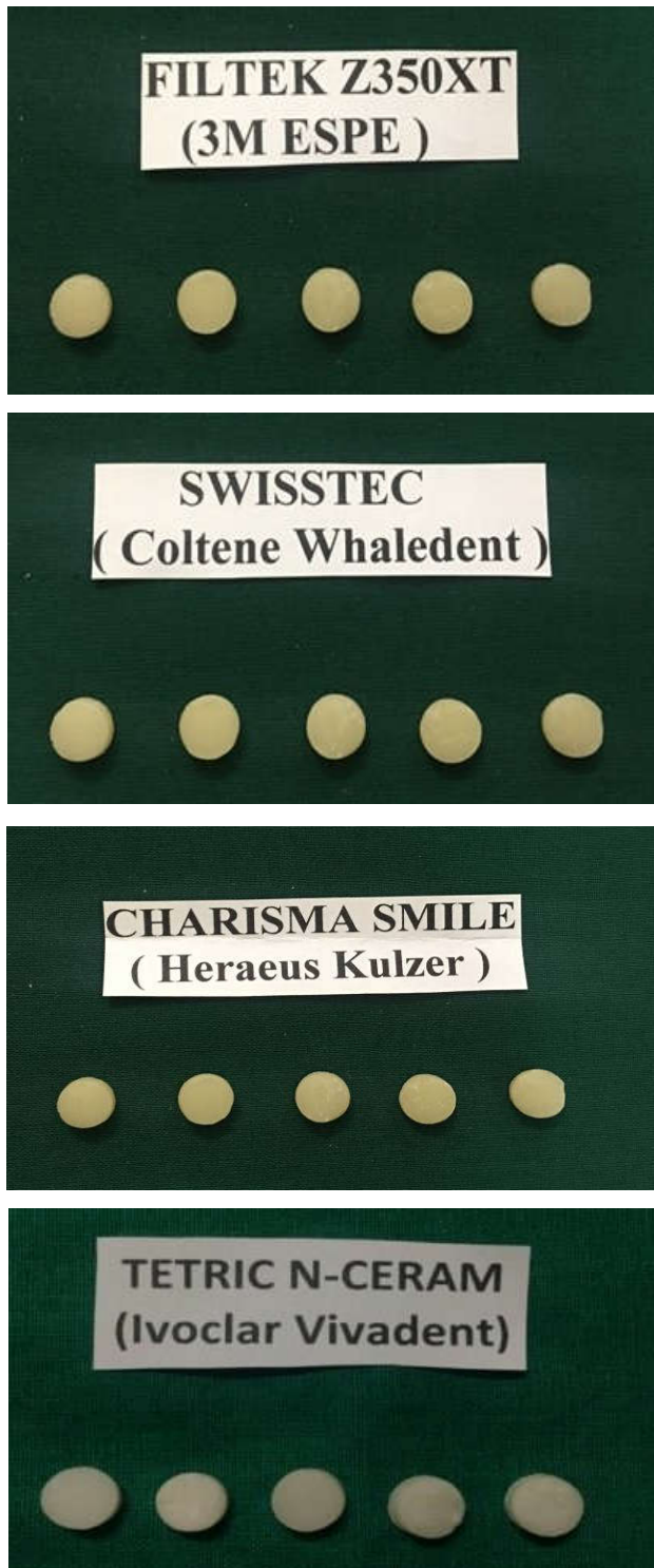
Fig 3 Disc shaped specimens of four resin composites
