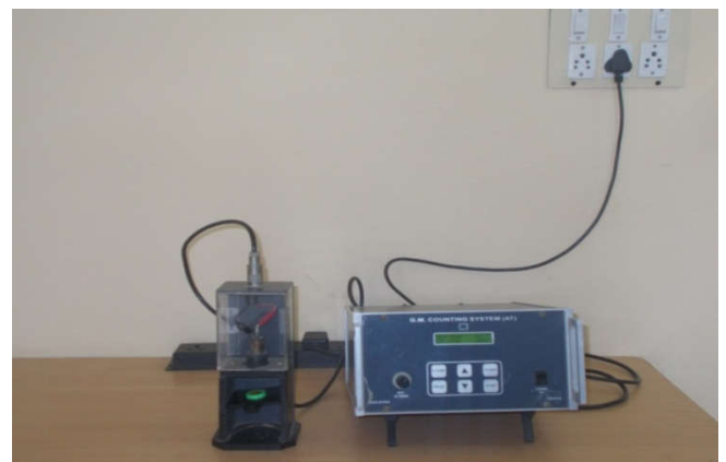
Fig 2 Experimental arrangement of G.M.Counting System
