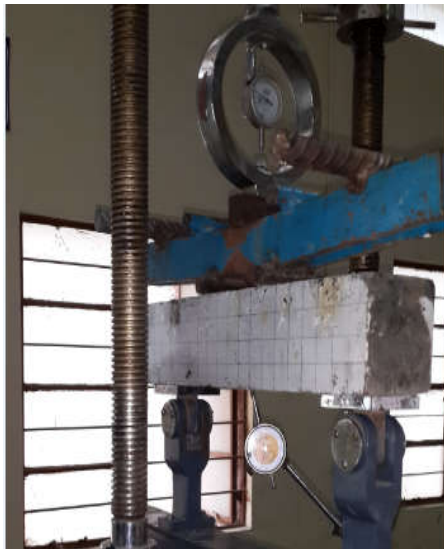
Fig.5 Deflectometer set up
