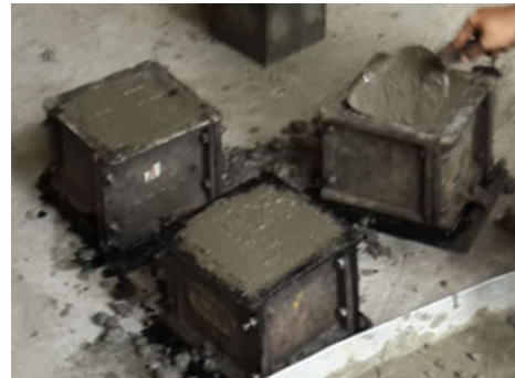
Fig.3 cube mould after concreting
