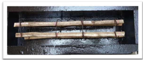
Fig.2 Beammould with bamboo Reinforcement
