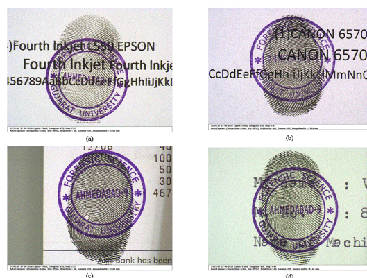
Figure 1 (a) Inkjet group (b) Laser group (c) Thermal group (d) typewriter group -Simulated overlapped of printed text, seal impression and thumb print
