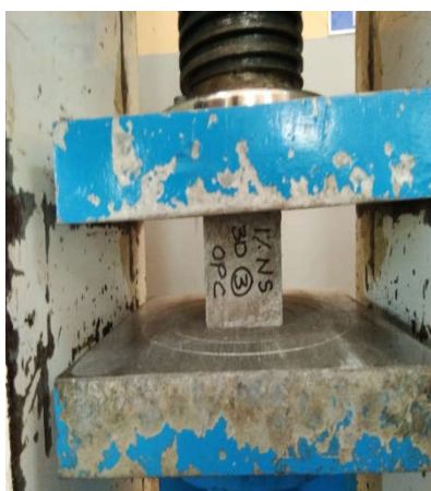
Fig 3 Testing of cube specimen
