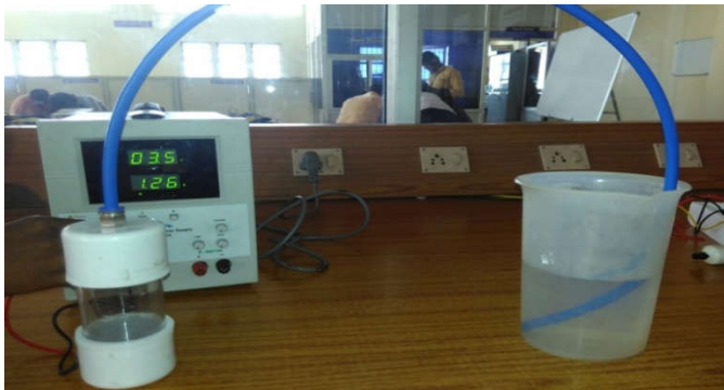
Fig 2 A photo of the tested HHO generator
