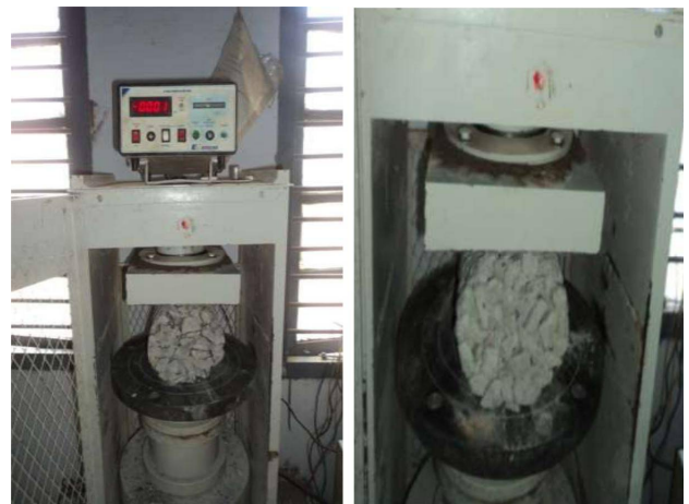
Fig 4 Testing of cylinder for Split Tensile Strength
