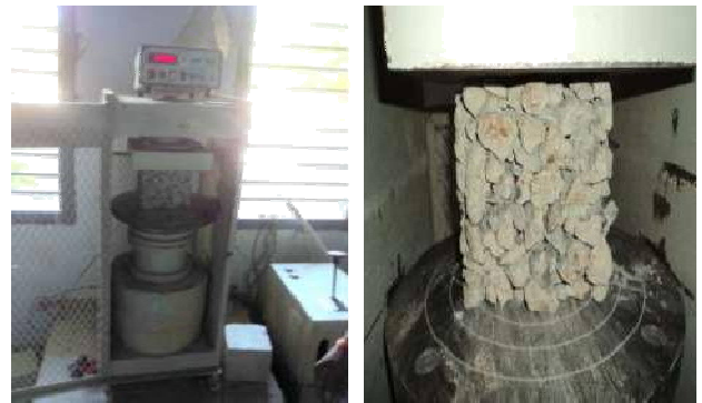
Fig 2 Testing of Cube
