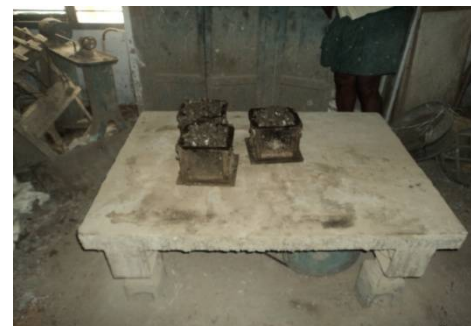
Fig 2 Mixing and compacting the specimens on table vibrator
