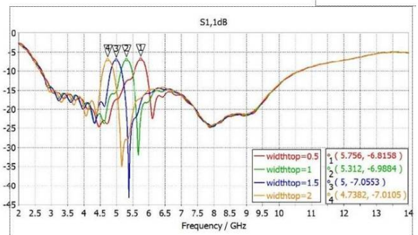
Figure 7 Parametric study of return loss for UWB monopole antenna with modified U-shaped SRR (with parametric study of SRR ring top width, W_{ringtop} )
