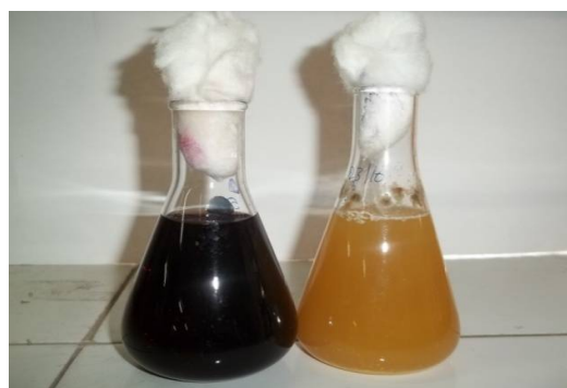
Fig 2 BDM containing RBB (100ppm) and medium decolorized by bacterial culture CS 2a4 under static condition at 37°C.
