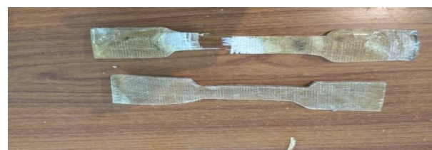
Fig 3 Showing the specimen before and after tensile test
