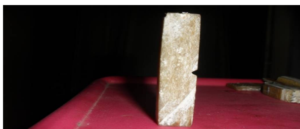
Fig 6 Specimen before impact test
