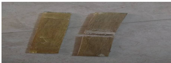
Fig 4 Showing the specimen before and after flexural test
