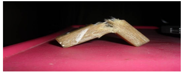
Fig 7 Specimen after impact test
