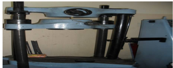
Fig 2 UTM for tensile test
