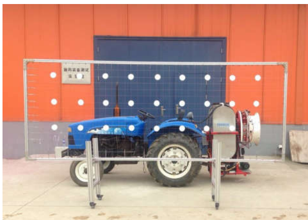
Figure 3 The layout of the collecting points in the test on the collecting device
