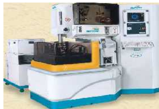
Figure 2 WEDM Electronica Elpuls 40ADLX [Wikipedia]
