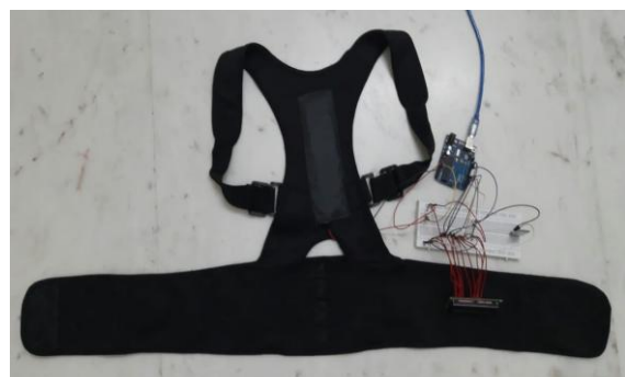
Fig. 11 Prototype of spine brace band integrated with flex sensor.
