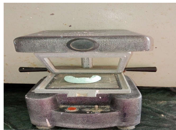
Figure 5 Vacuum pressing procedure
