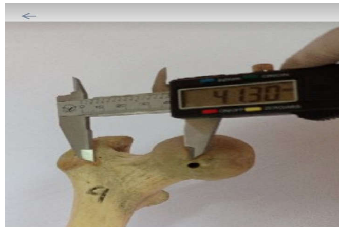
Fig 3 Femoral Horizontal offset measured by digital caliper
