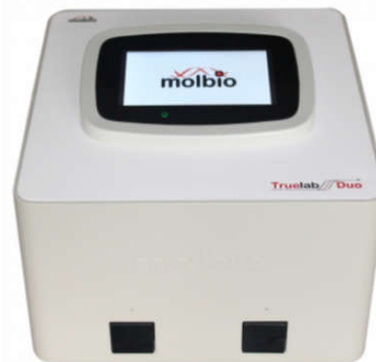
Fig 3 Truelab® Duo Real Time Quantitative micro PCR Analyzer
