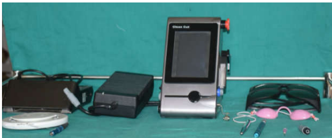
Figure 1 Dental surgical diode laser 980 nm (DENLASE 980nm/7)
