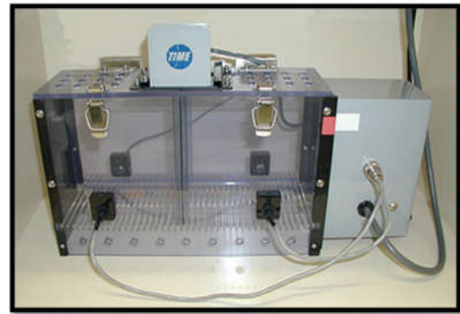
Fig.6 The Active Avoidance apparatus (shuttle box), divided in to two chambers
