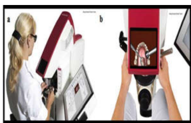
Figure 2: (a) MOOG Simodont Dental Trainer (adapted from www.moog.com); (b) A haptic tooth preparation exercise.
