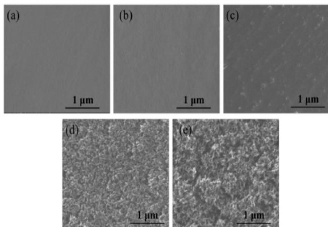
Figure 9 SEM images of un-modified (a), and modified PEGylated surfaces with different CF<sub>4</sub> plasma treatment time (b) 2.5 min, (c) 5 min and (e) 10 min<sup>23</sup>
