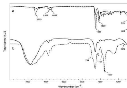
Figure 7 (a) ATR-FTIR spectra of PA66 fabric and (b) FTIR spectra of the aqueous extraction residue after blank dyeing process. With plasma (dotted lines) and without plasma (solid lines)<sup>18</sup>.
