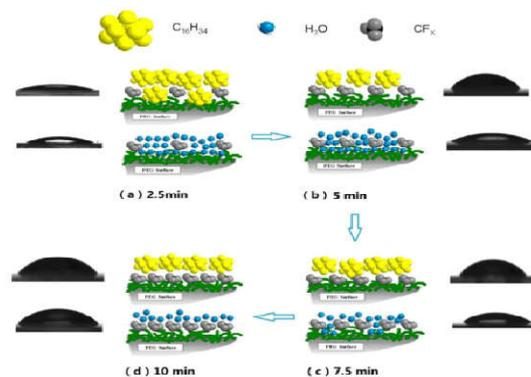
Figure 10 Schematic representation of wetting mechanism of the modified PEGylated Surfaces with different CF<sub>4</sub> plasma treatment<sup>23</sup>
