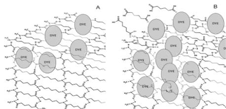
Figure 6 Dyeing mechanism of nylon 66 fiber before (A) and after (B) plasma treatment<sup>18</sup>.
