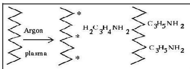
Figure 5 Grafting of a monomer on the surface<sup>12</sup>
