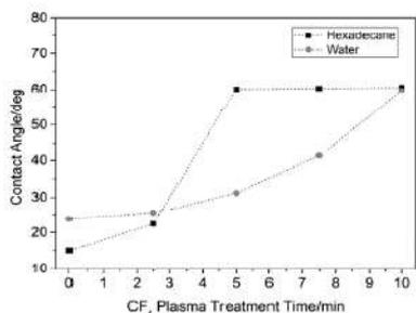
Figure 8 Contact angle measurements of water and hexadecane on the modified PEGylated surfaces with CF<sub>4</sub> plasma treatment time<sup>23</sup>.
