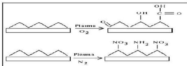
Figure 4 Surface activation by substituting hydrogen in a polymeric chain with other groups (O, OH, COOH, NO<sub>3</sub>, NH<sub>2</sub>, etc.)<sup>12</sup>
