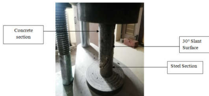
Figure 2 Testing of Slant Shear Bond
