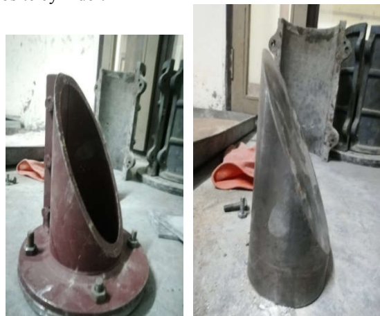
Figure 1 concrete mold and steel specimen for SST
