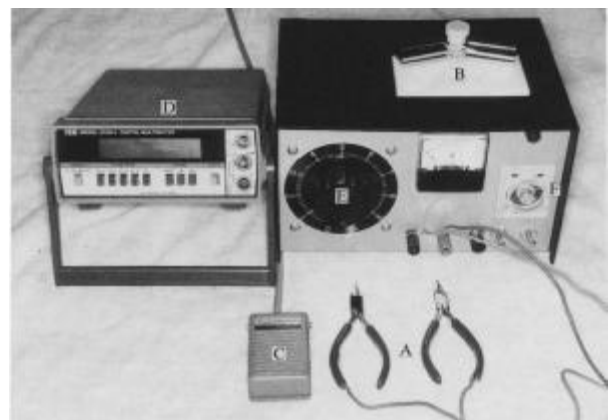
Figure 17 The equipment for DERHT method, (a) electric pliers, (b) electric arch holder, (c) foot switch, (d) electric current meter, (e) transformer, (f) timer. 15
