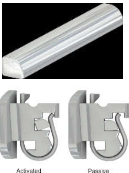
Figure 10 Any rotation of the bracket relative to the wire, away from the relationship shown on the left, results in labial deflection of the Spring Clip and thereby storage of appropriate energy for recovery. This relentless homing action enables precise tooth positioning in all planes of space.
