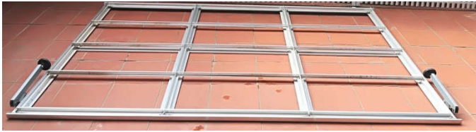
Figure 3 Alluminium chassis embedding the 12 rectangular double-chamber PVC panels (see Fig. 2).
