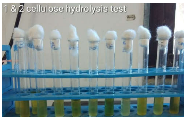
Fig 2 Cellulose hydrolysis test using CMC and bromothymol blue.
