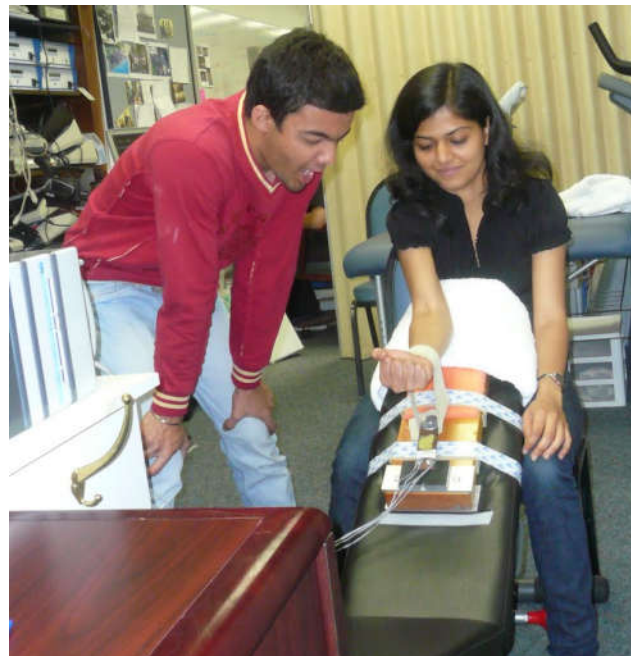
Figure 1 A typical subject setup for the repetition maximum (RM) and muscle strength (MS) measurements while the examiner is giving verbal cues. Also seen here is the strain gauge device with the wrist strap, securely attached to the 45° angled bench.
