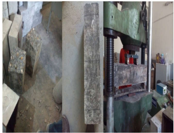
Photo I Flexural Strength Test of Beam Specimen
