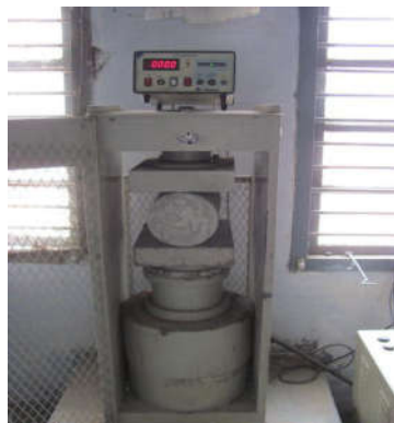
Fig 2 Split Tensile Test Setup
