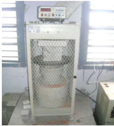
Fig 1 Compressive Strength Test Setup
