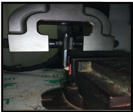
Figure 2 Specimen mounted and shear bond strength testing done on a Universal Testing machine.
