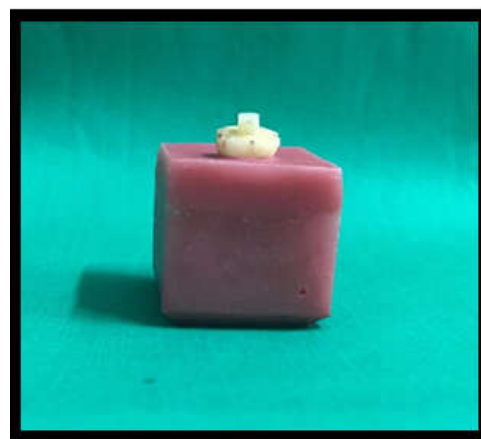
Figure 1 Representative image of prepared specimen for shear bond strength testing
