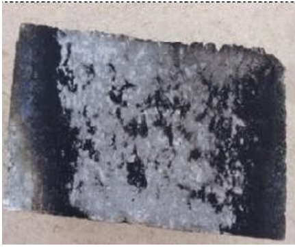
Fig 7 Papercrete after fire test
